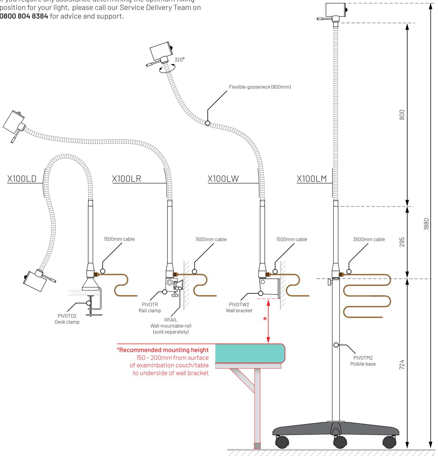
All measurements in millimetres (unless otherwise stated)
